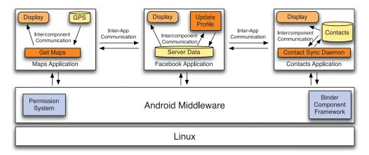
Fig. 1. How Android application components interact within the same app, with other apps, and with the Android framework.
